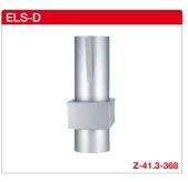
Fire protection ceiling seal ELS-D to prevent spread of fire to other floors. Installation in main ventilation pipe according to DIN 18017 K90. Maintenance-free. For ventilation or mixed (even with combustible pipes) installation shafts which only require cladding with 12.5 mm
