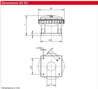
Extremely weather-resistant EC roof fan in plastic design for an extensive range of applications, diagonal outlet.
