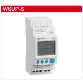
WSUP-S Ref. no. 09577 Digital timer with illuminated LCD display for automatic controlling the operating modes of any units up to 16 A rated current. Suitable for switching the smallest electric currents from 1mW (0.1V/1mA) through standard, gold-plated  $\mu$  contact. 56 programmable switching times for all weekdays. With smartphone via NFC (free App).
