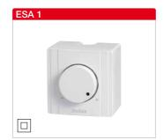
ESA 1 Ref. no. 00238 Max. load 1 A White plastic casing, operation indicator via light ring in rotary knob. Minimum load 0.15 A Protection category IP40 Wiring diagram no. 556.1 W 80 x H 80 x D 65 Dim. mm
