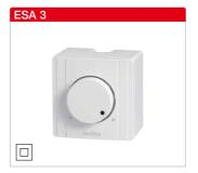
Ref. no. 00239 ESA 3 Max. load 2.5 A (T 40 E) White plastic casing, operation indicator via light ring in rotary knob. Minimum load 0.15 A
