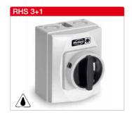
RHS 3+1 Ref. no. 01594 "0" position can be locked with a padlock. In accordance with DIN EN 60204 p.1/VDE 0113-1. Plastic casing for surface-mounted installation. 3-pole with auxiliary contact, for single-speed and speed-controlled fans.
