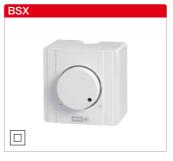
**BSX** Ref. no. 00240 Max. load 1 A (T 40 E) Surface-mounted speed controller with reverser for reversible fans (supply and extract ventilation) in white plastic casing. Only for fans which are reversible using a changeover switch.
