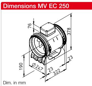
**Energy-saving EC round duct fan with high pressure performance, high volume output and space-saving dimensions.**
