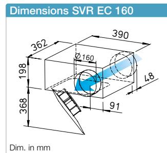
**Energy-saving EC circular duct fans for the delivery medium and small air volumes against high resistances.**
