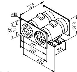
rated mounting bracket by loosening the clamp. All components are made of impact-resistant and corrosion-resistant plastic. Colour: Light grey.
