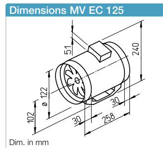
**Energy-saving EC round duct fan with high pressure performance, high volume output and space-saving dimensions.**
