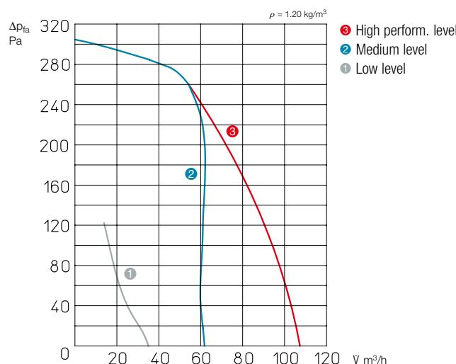
\* Char. curve with factory connector position.
