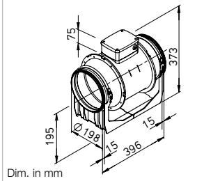
**Energy-saving EC round duct fan with high pressure performance, high volume output and space-saving dimensions.**
