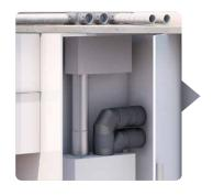
The **duct system for the extract air** is realised using the FRS flexible ducts set into the concrete floor. Thus, all ventilation lines are invisible in the building structure. Only the ventilation unit and the distribution boxes have inspection openings for simple maintenance.
